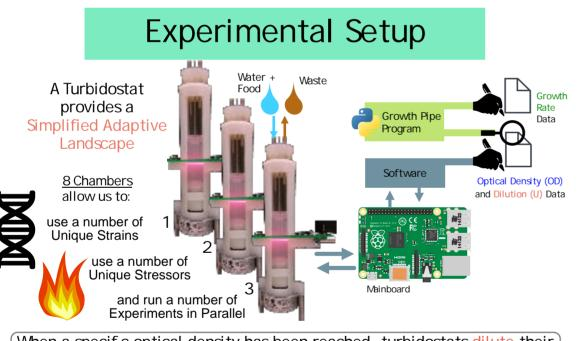
When a specific optical density has been reached, turbidostats dilute their growth chamber, **removing** some solution and **adding** some food and water. This decreases common stresses that microorganisms often adapt to such as high cell density, waste saturation, and limiting resources.
